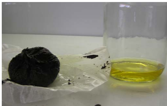
Dewatered Sludge and filtrate
