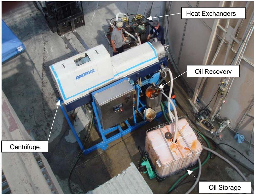
The solids generated 7 fork lift bins of sludge over an 8 hour period and was dumped into the garbage dumpster for local landfill disposal. The oil split generated 275 gallons of oil (76% purity) over the days test. The volume reduction was the difference in sludge feed at 10 gpm which was reduced to 1.5 gpm in dewatered sludge dropping from the centrifuge or an overall volume reduction of 85%. This exceeded the required 4:1 reduction or 75%.
