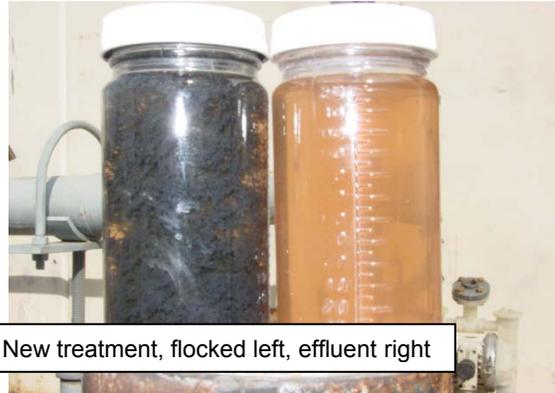
New treatment, flocked left, effluent right
