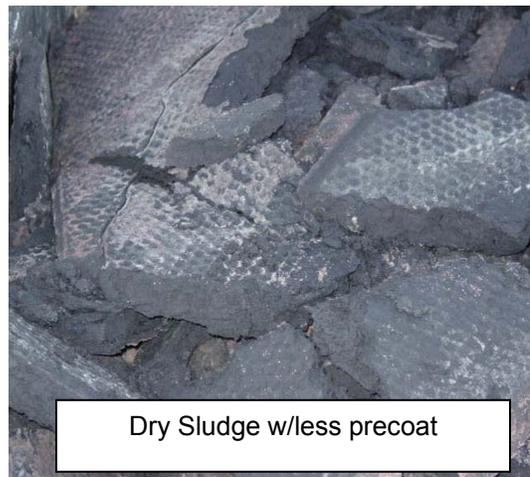
Dry Sludge w/less precoat
