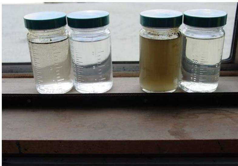
The lower photo has Tank 31 untreated and treated on the left 2 jars and Tank # 3 untreated and treated on the right. Analytical samples were taken and sent to the lab for testing of Oil & Grease as well as COD for both untreated and treated samples. The analytical samples were received by the lab, but unfortunately they made a mistake in the testing procedures so there were no results to report.
