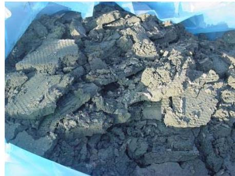
The facility was having varied and unstable pH and conductivity levels. The variable pH, due to starch dumps, was causing irregular treatment of the water. The sludge was not dewatering fast enough, backing up the water in the system. To remedy this, the facility required the treatment tank to be pumped out weekly and have the sludge hauled off site wet at a cost of \$4,000/load.
