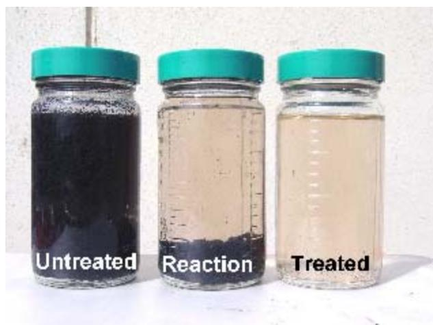
The chemicals are added and the flocculated wastewater is allowed to settle and switches to the dewatering step. The dewatering step involves the addition of 1-1/2 bags of diatomaceous earth as a filter pre-coat (helps the sludge cake release from the plates as well as a filter enhancer) and then the treated batch is pumped to the Filter Press. The Filter Press acts as a filter, filtering the wastewater which then goes to the Treated Water Tank as well as dewateres the sludge.
